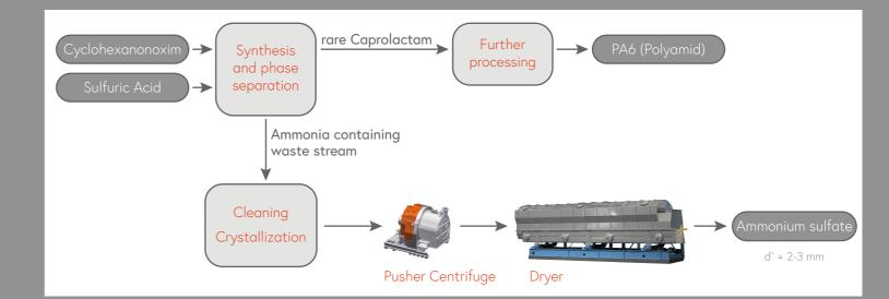
2) Synthetic production of ammonium sulfate out of ammonia gas and sulfuric acid.
